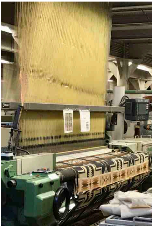
The yarn spindles feeding the weaving machines are actually located in the floor above where the machine is located.
